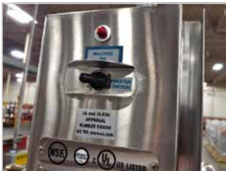
Master switch with control light above
