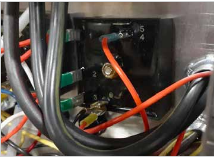
Motor contactors and overloads attached
