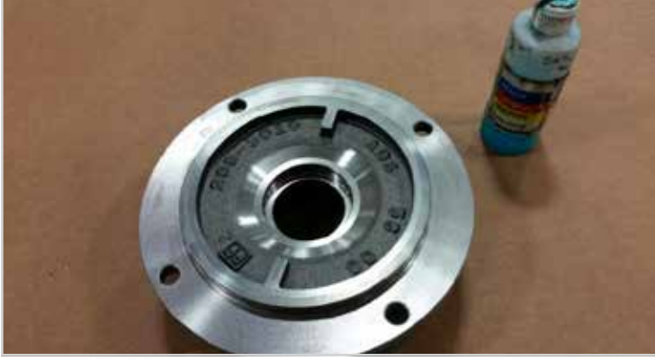
Lubricate the pump housing with some dish soap
