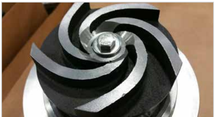
Key in the keyway, place impeller & tighten lock bolt 15 ft/lbs
