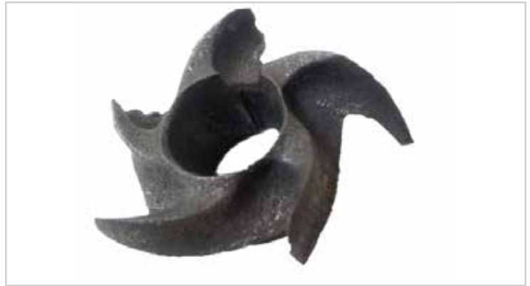
Result of spinning impeller in high ratio acid solution
