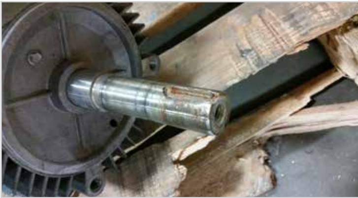
Showing key way damaged
