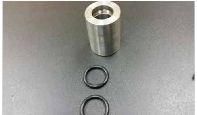
Motor shaft sleeve w/inner o-rings
