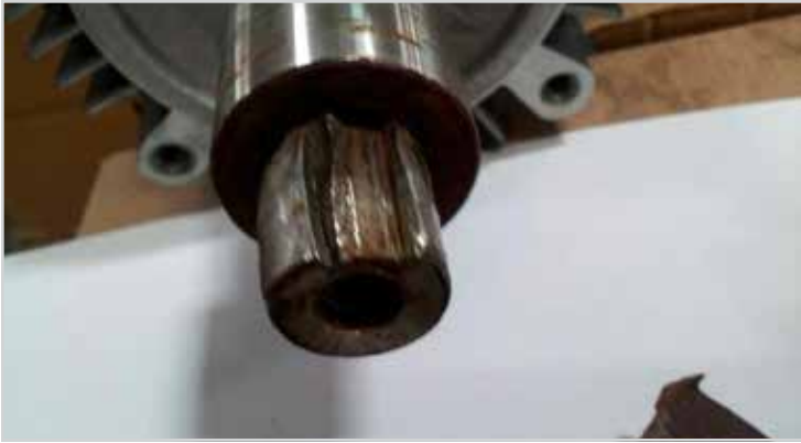
Motor with damaged key way
