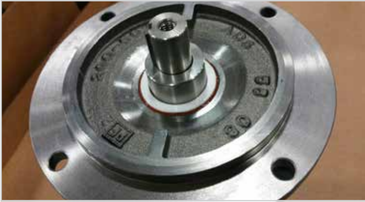
Press the ceramic half of the seal w/boot into the housing
