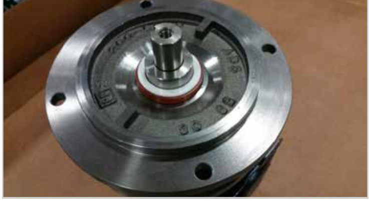
Place the housing on the motor w/sleeve installed
