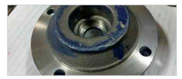
Now with the aux shaft attached, place the pump housing (282-6307) to the motor.
