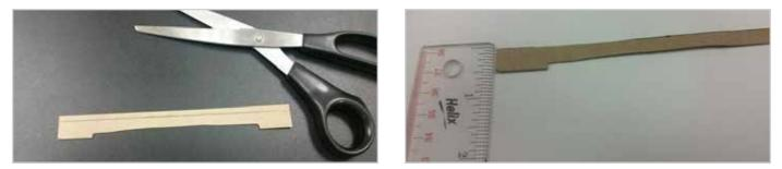
In the field, a gauge can be made by cutting a template from cardboard and use it to mark the shaft.
