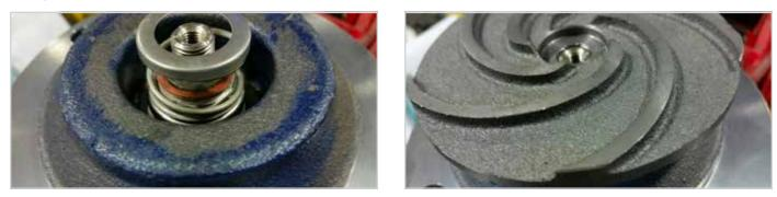
Place the black graphite half on the shaft and press until it is touching the white ceramic half. Use soap to lubricate the inside of the black rubber half. Be careful with this operation, the ceramic portion is glass and can break when blows are laid against parts of the pump.
