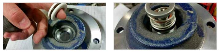
Then place the ceramic half of the seal in the housing, use soap to lubricate and press in to the bottom. The groove side will face down or towards the motor side.
