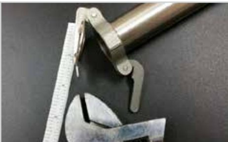
Will not stay closed the tab is bent inward
