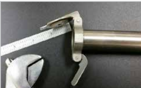
Correct alignment of tab is straight with the cap
