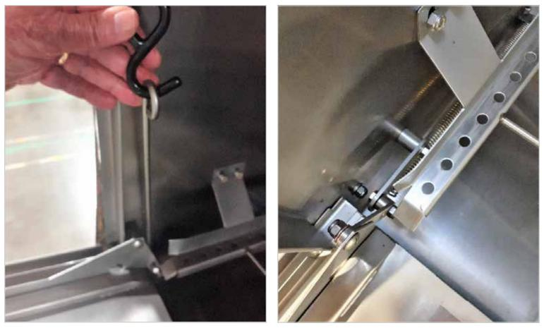
Then using the ratchet, draw the link upward until the hole of the link and the hole on the door rail align. When tightening the bolt, make sure that 1 to 2 threads are showing through the lock nut.
