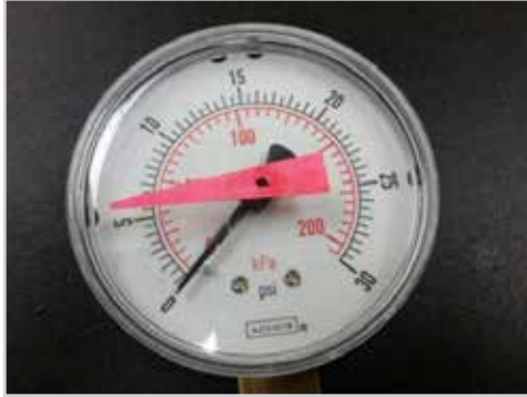
Lower wash arm pressure approx 5-6 psi
