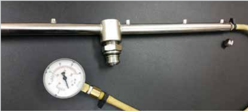
088-1048, Tool, Spray Arm with pressure gauge for low temp machines
