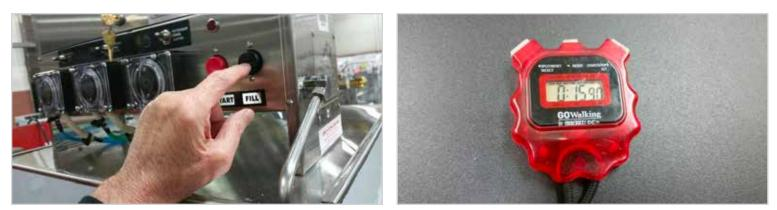
Second: While pushing the fill button, count the seconds it takes to refill the machine.
