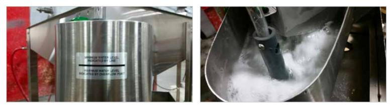
**Third**: The water level decal indicates the approx fill level. Release the fill button when this level is reached. Record the seconds it took to reach the fill level.
