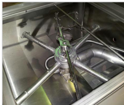
Final rinse arm twisted into transfer tube
