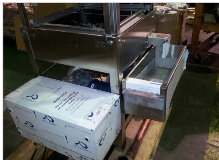
Showing built-on booster mounted in corner position (front)
