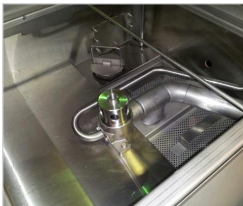
Showing spray arm base & transfer tube
