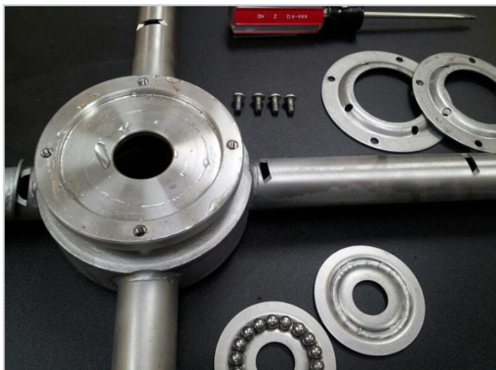
Races are interchangeable, capture shells are also
