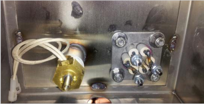
Showing thermostat and sustainer heater terminals*
