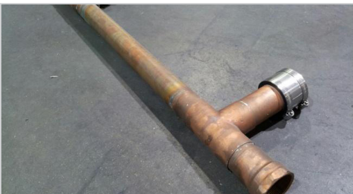
HT-25 drain manifold with "no-hub" connectors
