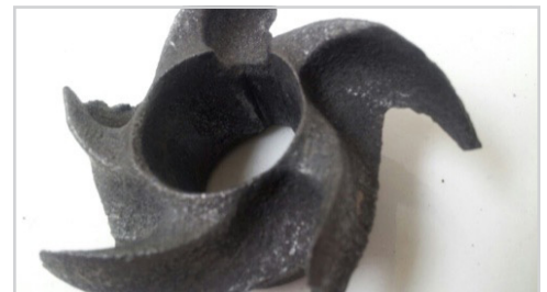
Impeller damaged from high acid solution
