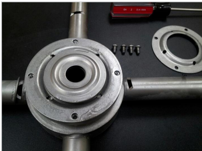
Remove top shell, exposing top bearing race
