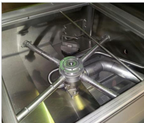
Wash arm w/bearing installed on base
