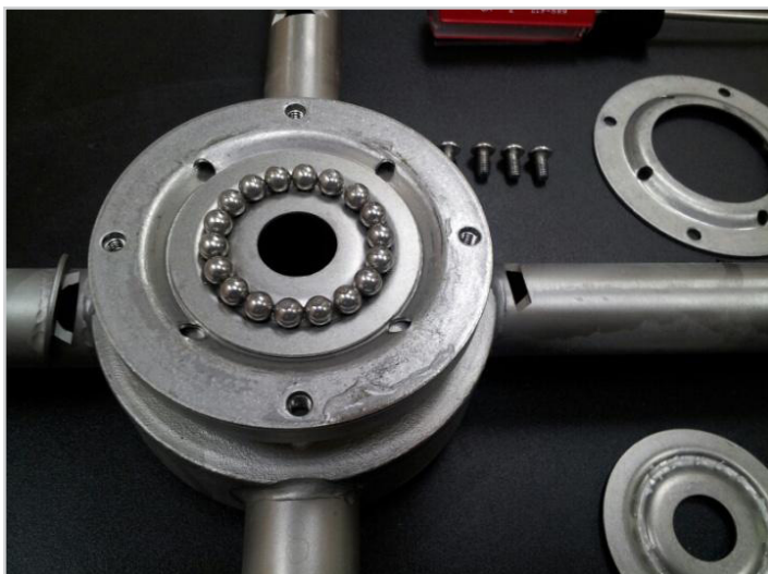
Top race removed, ball bearings for replacement
