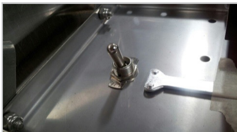
De-lime switch in HT-25 control box
