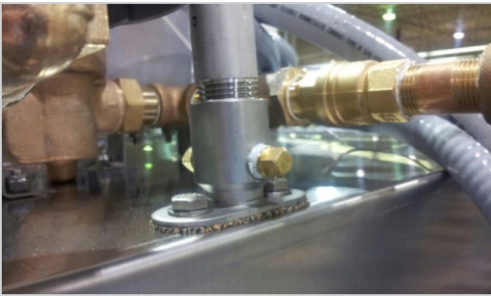
Mixing chamber with two 1/8" pipe threaded port
