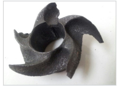
Impeller damaged from high acid solution
