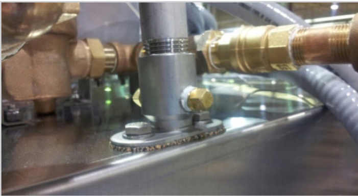
Mixing chamber with two 1/8" pipe threaded port
