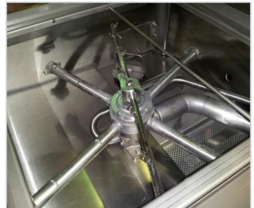
Final rinse arm twisted into transfer tube
