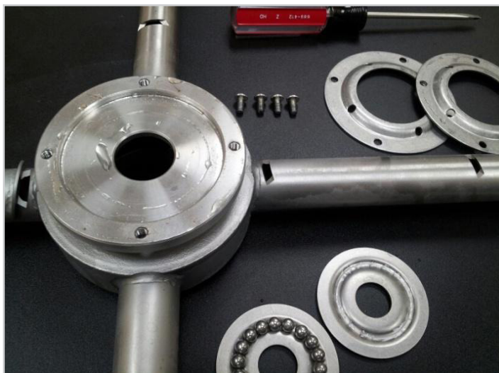
Races are interchangeable, capture shells are also
