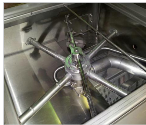
Final rinse arm twisted into transfer tube
