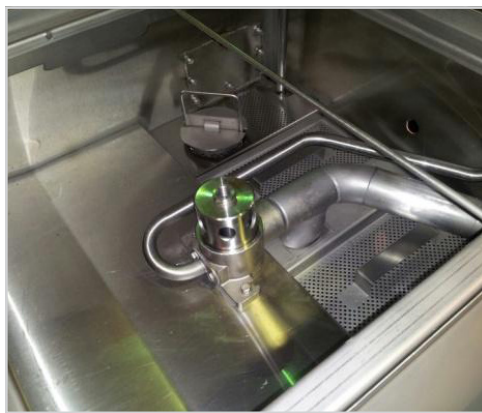
Showing spray arm base & transfer tube
