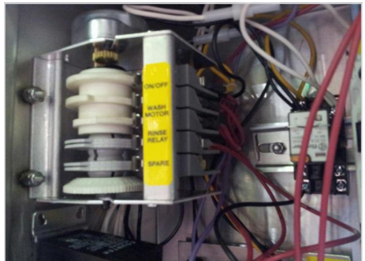
Cam timer with 3 fixed operational cams, 2 adjustable
