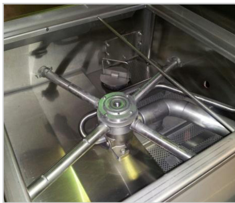
Wash arm w/bearing installed on base
