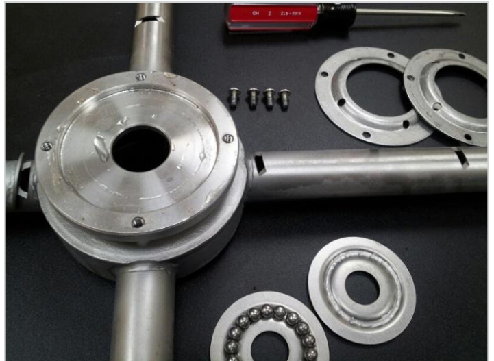
Races are interchangeable, capture shells are also
