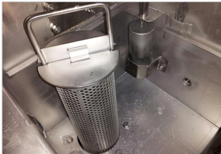
Pump filter in drain sump
