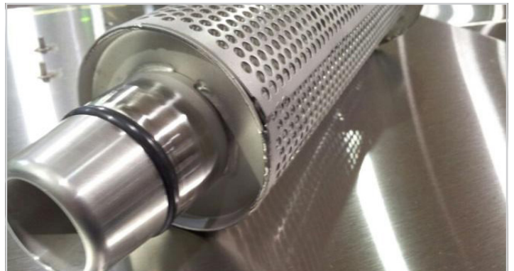
Pump filter and drain plug, note O-ring seal
