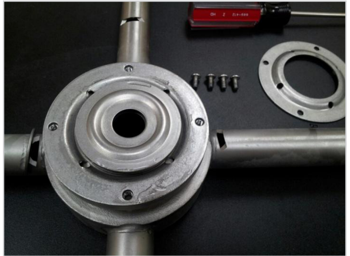
Remove top shell, exposing top bearing race
