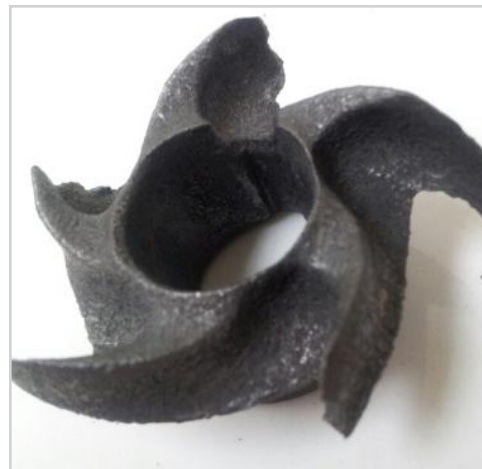
Impeller damaged from high acid solution
