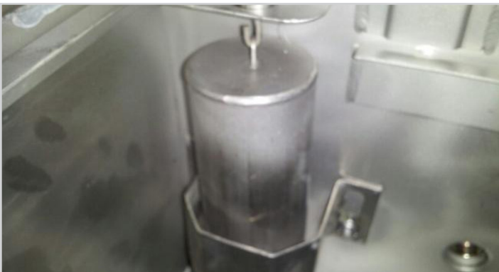
Wash tank float and tank overflow
