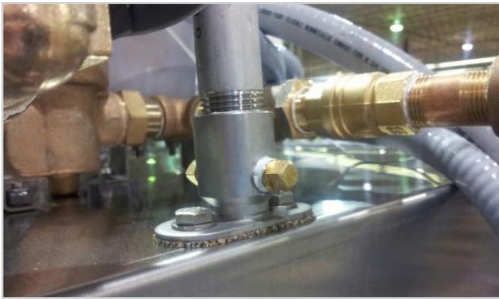
Mixing chamber with two 1/8" pipe threaded port
