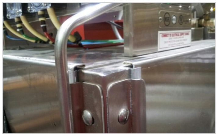
Showing correct arm alignment
