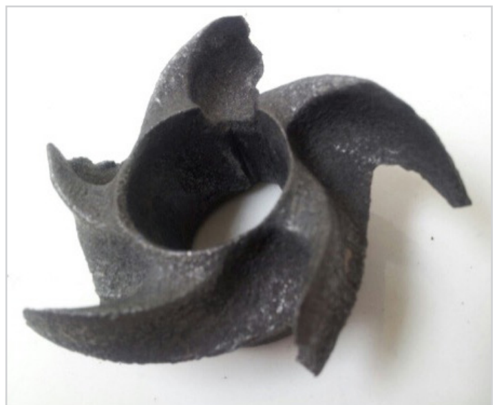
Impeller damaged from high acid solution
