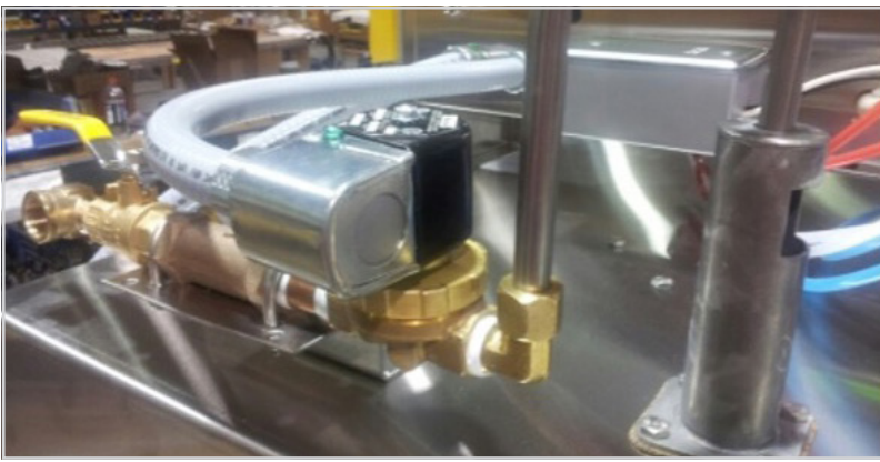
Showing 1/2" female pipe inlet, ball valve, y-line filter, water solenoid, ASSE approved air gap (backflow preventer)
