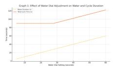
This graph illustrates the relationship between the water dial setting, the resulting Water Duration, and how it affects the Total Cycle Time:
