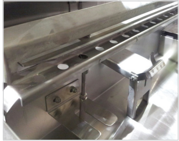
Wash tank sequence bar, pendulum with magnet
