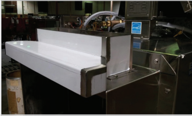
Vent attachments to end shield, 4" x 16" opening
