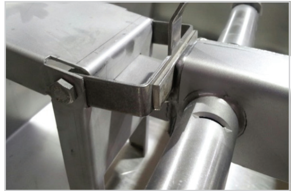
Arm resting in "T" index with latch down
