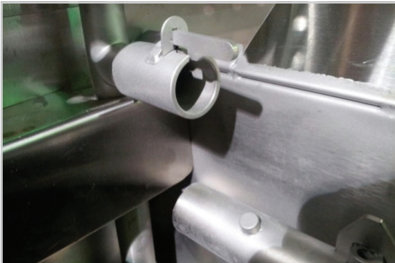
Showing pumped rinse manifold locking tab
