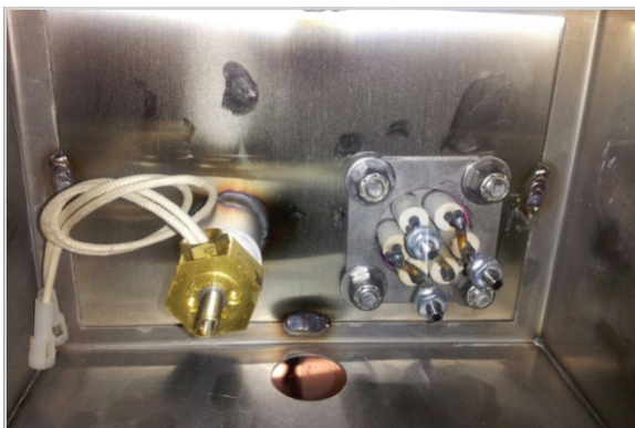
Wash tank thermostat, rotate center rod Left to increase
