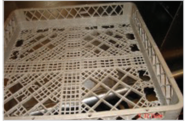
Damaged and broken rack that will jam or skip conveyor
