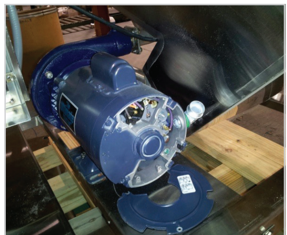
66 power scrapper motor, 1.5 HP, 208v, single-phase
