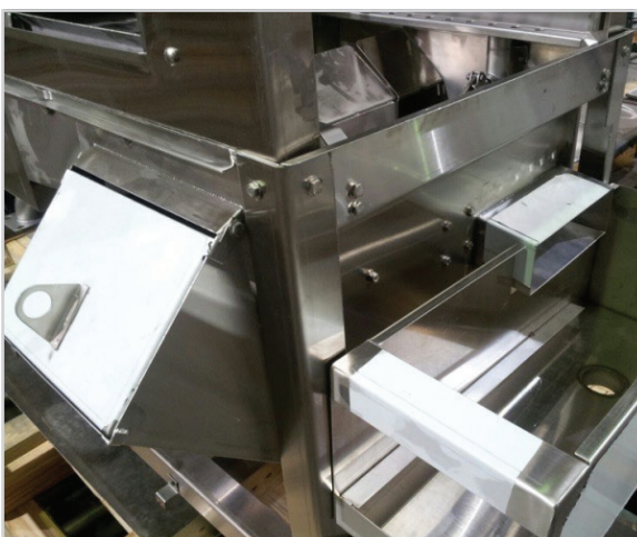
ADC-66 power scrapper, overflow to scrap box
