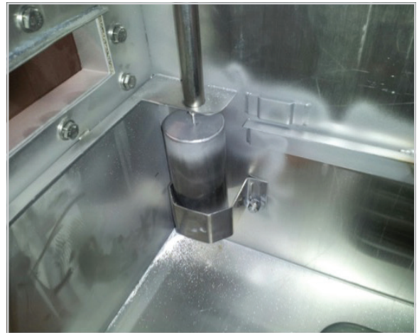
Wash tank float and tank overflow
