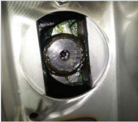
Cam bearing screws into cam block B
