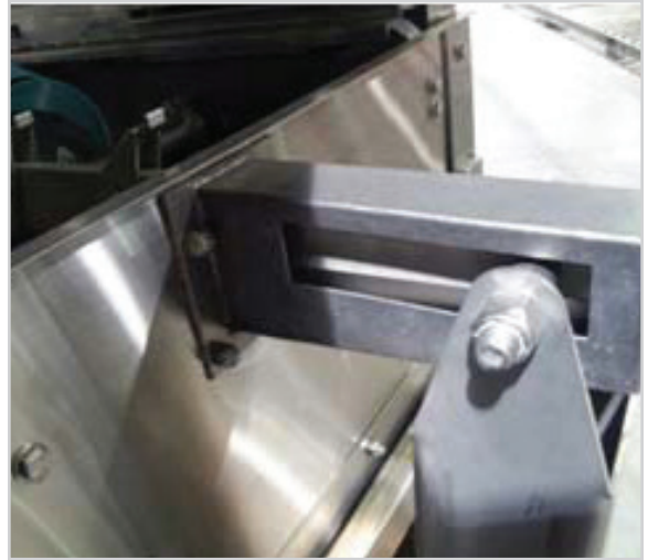
Rocker arm attached to conveyor bar, drip chute
