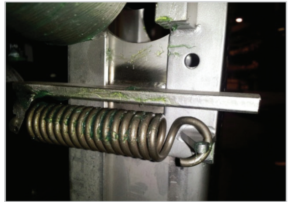
Rocker arm slip clutch spring, hook to bar weldment
