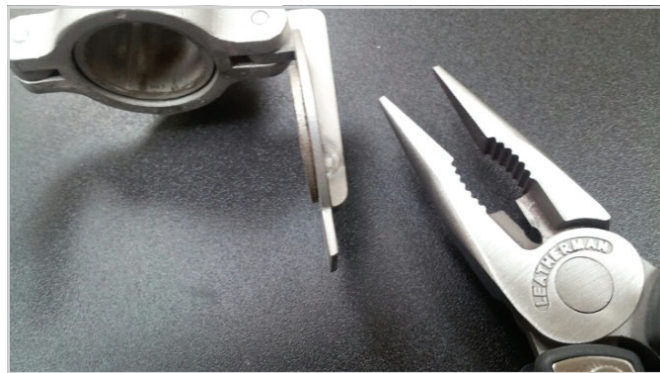
Straighten tab in line with the coin edge to tighten latch
