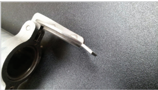
Tab on endcap bent inward, causing loose fit
